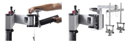
The electrical lifting axis is controlled by a joystick and makes for comfortable operation. There are storage locations for two grinding wheels and up to three clamping arbours. Furthermore, a generously dimensioned tooling drawer and the integrated grinding wheel setup device turn the ErgoMount into a convenient helper in every production environment.
