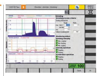
of time signals captured by the measuring sensors. The monitoring system's scalar format for the data parameters makes graphical representation easy, even with thousands of measured datapoints. Moreover, the system does not require specific evaluation software and hardware, and can be operated with a simple web application on standard web browsers.
