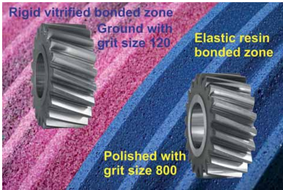
Fig 1: Direct comparison between the ground (left) and the polished ground (right) gear.
