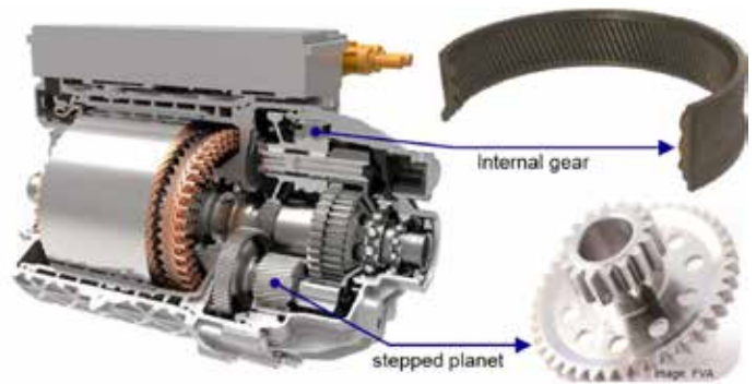
Figure 1: Left: Motor gear unit of a modern traction drive [2]. Right: Examples of internal gear and a stepped planet.
