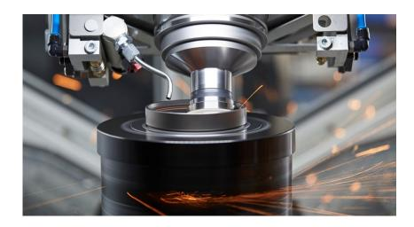
gear skiving process. In high-volume production, the thermal stability of the process and machine is crucial. One of the main development goals of the machine was therefore thermal symmetry, which ensures the highest dimensional accuracy across the entire batch.
