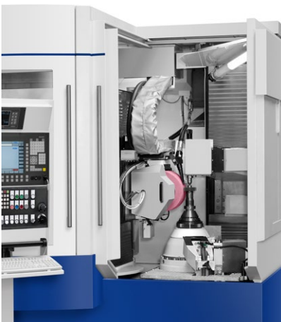
Optimum accessibility: Grinding position, wheel changing position, dressing position
