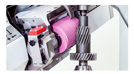
The upgrade module for the Reishauer RZ 410 to RZ 1000 uses a corundum grinding worm, reduced in diameter to  $140\,\mathrm{mm}$  (d<sub>f min</sub>  $67\,\mathrm{mm}$ ), making the advantages of the generating grinding process available for extended applications. It thus fills the gap between our highly productive RZ 126/160 KWS 4.0 twin-spindle models and the profile grinding process.
