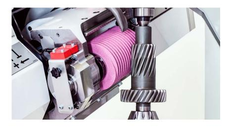
The upgrade module for the Reishauer RZ 410 to RZ 1000 uses a corundum grinding worm, reduced in diameter to 140 mm (d<sub>f min</sub> 67 mm), making the advantages of the generating grinding process available for extended applications. It thus fills the gap between our highly productive RZ 126/160 KWS 4.0 twin-spindle models and the profile grinding process.
