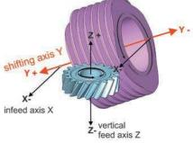
Figure 2: Continuous generating grinding axis motions
