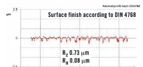
Figure 12: Surface finish on polish-ground gear
