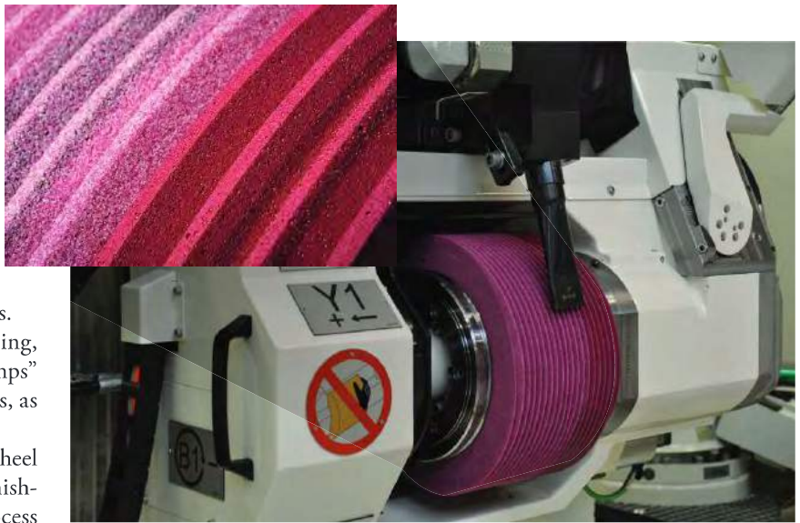
Figure 3: Two-zone threaded grinding wheel
