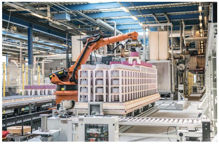
Illustration 5: Robot loading of a kiln cart
