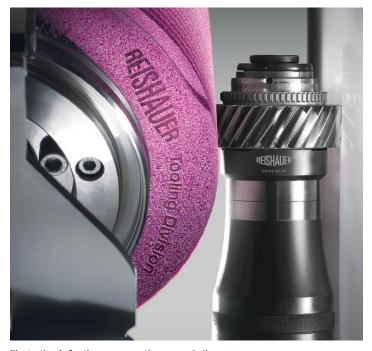
Illustration 1: Continuous generating gear grinding process
