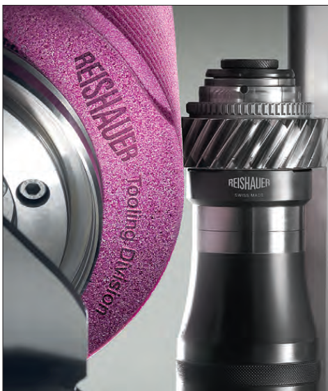
1-Continuous generating gear grinding process
