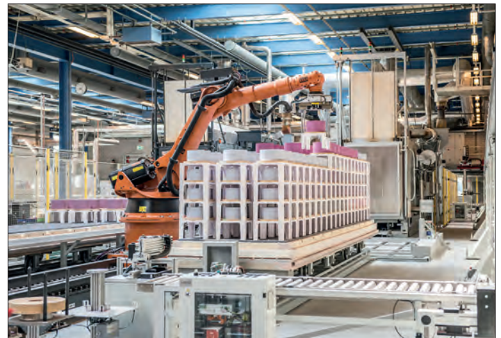
5-Robot loading of a kiln cart
