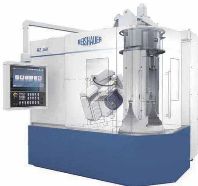
Reishauer RZ 260 twin-spindle generating gear grinder
