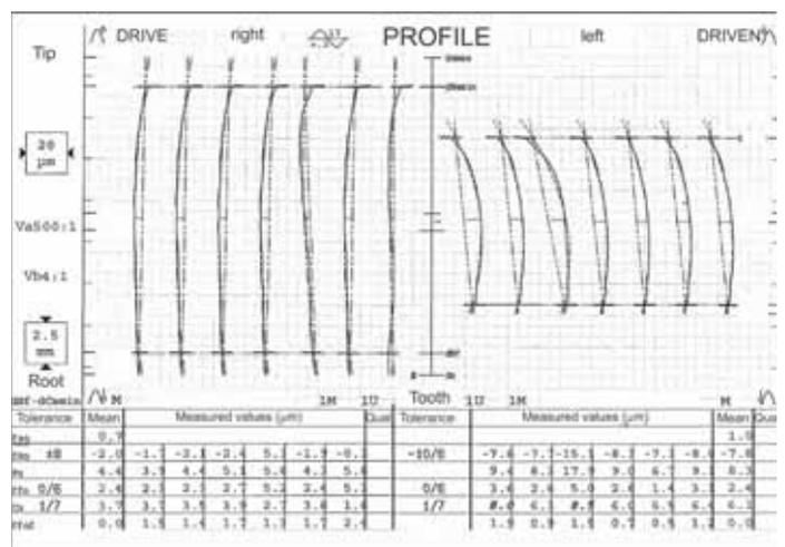
Illustration 6: Gear chart of ring gear profile
