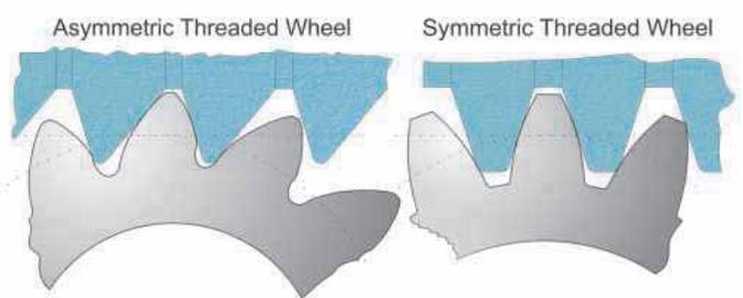
Illustration 3: Asymmetrical and symmetrical grinding wheel profiles
