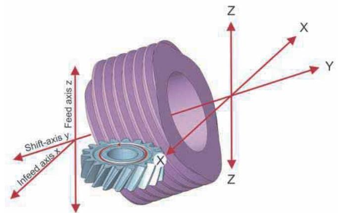
Illustration 2: Kinematics of the continuous generating process
