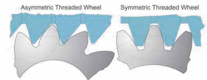
Illustration 3: Asymmetrical and symmetrical grinding wheel profiles
