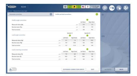
To visualize the results of the measurements, they can be accessed at the grinding machine in PDF form. This saves dealing with reports on paper, and also guarantees the correct machine and workpiece assignment. In addition, this visualization serves as a control function, supporting the operator in his decision about whether manual adjustments are required.
