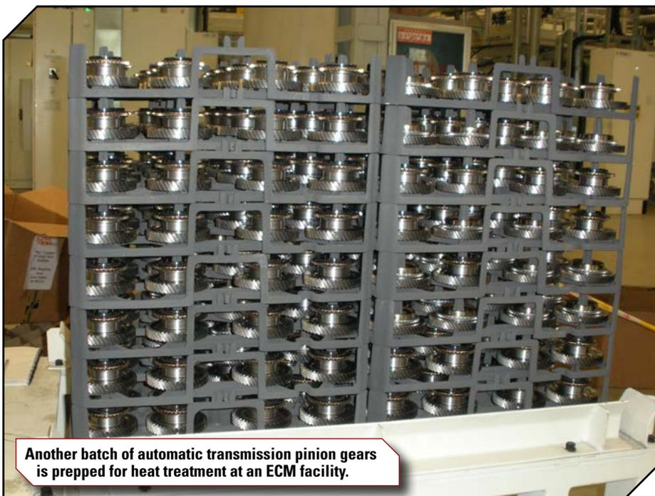
Another batch of automatic transmission pinion gears is prepped for heat treatment at an ECM facility.
