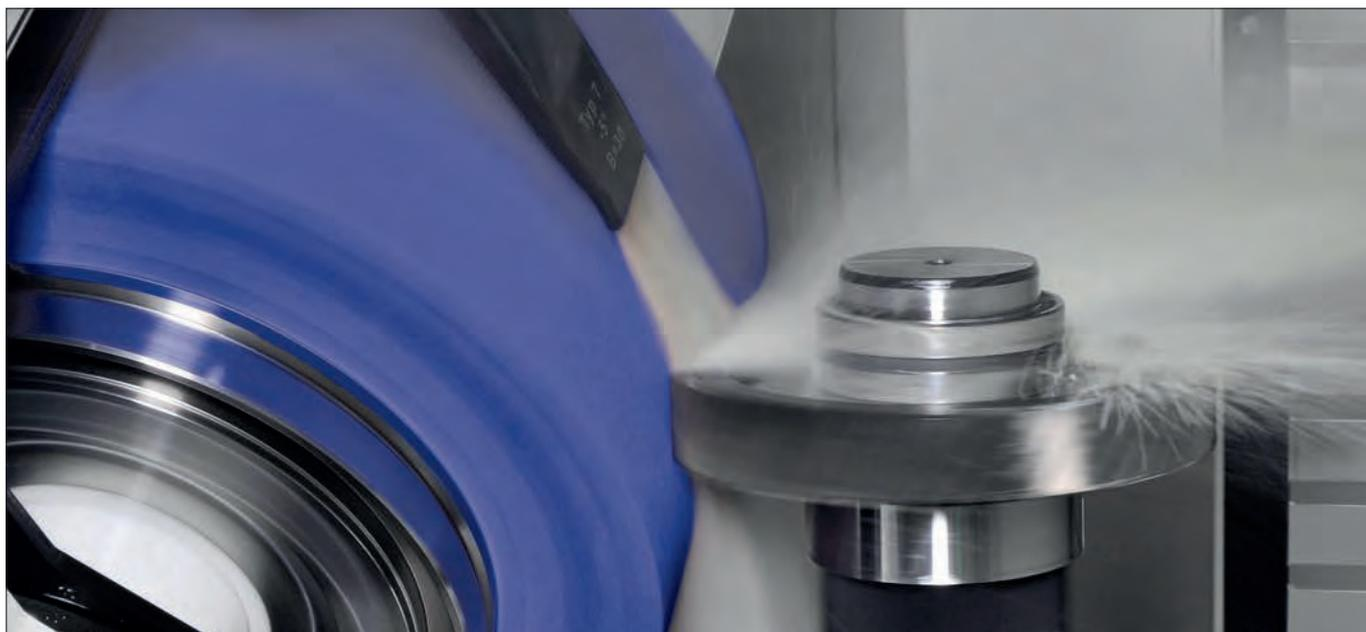
*Continuous generating gear grinding process in action*
