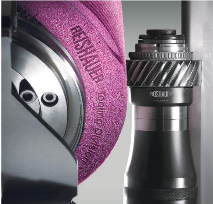
Illustration 1: Continuous generating gear grinding process
