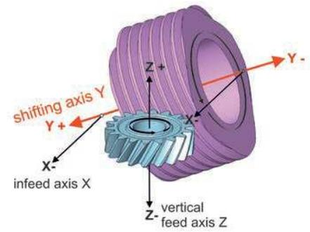
Figure 2: Continuous generating grinding axis motions
