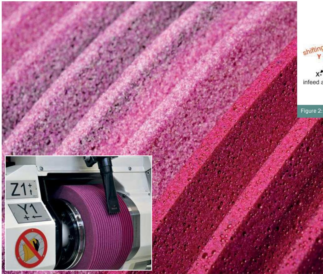
Figure 4: Two-zone grinding worm (grinding and polishing)
