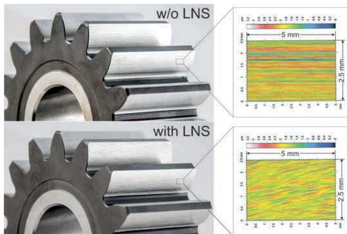
Figure 3: Surface structure without and with LNS
