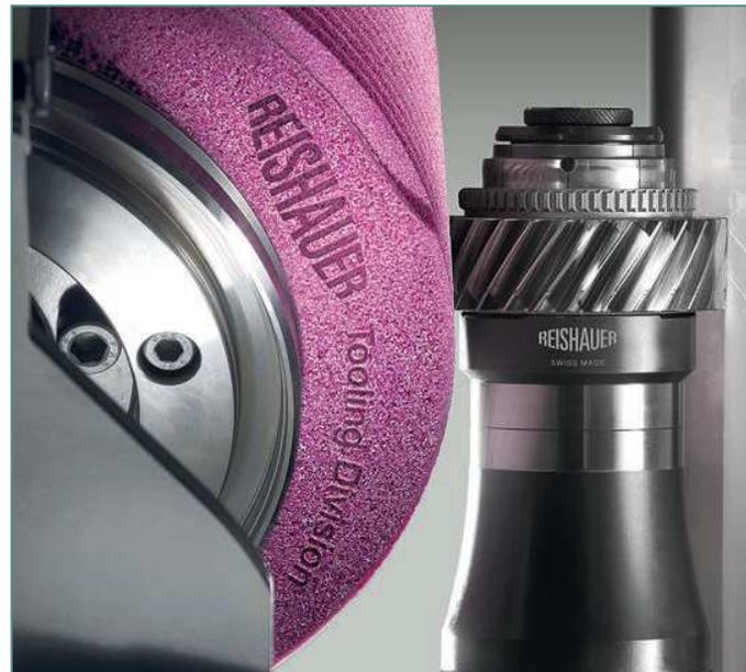
Figure 1: Continuous generating gear grinding
