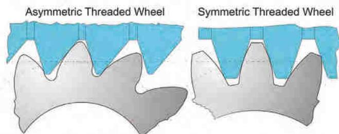
Figure 1: A depiction of both asymmetrical and symmetrical grinding wheel profiles
