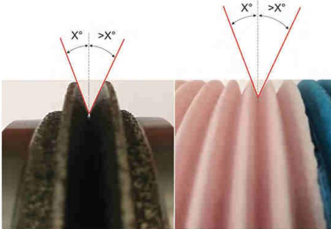
The asymmetrical diamond dressing roll (left) and asymmetrical threaded grinding and polishing wheel (right) enable greater efficiency and economy in gear grinding
