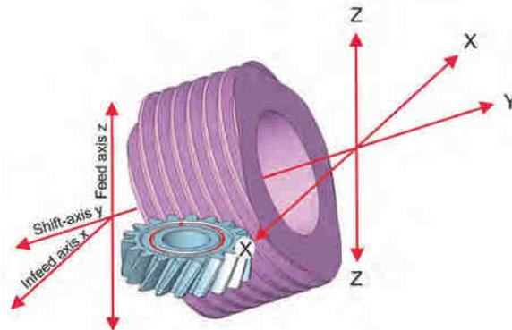
A kinematic diagram of the forces involved in the continuous generating process
