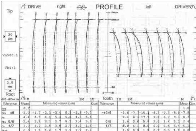
The results demonstrated from an asymmetrical ring gear, polish ground with gear data of 60 teeth, a module of 2.8 as well as a pressure angle of 30.5°/16.5°
