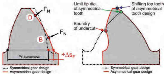
Figure 2: Features of asymmetrical tooth shape.  $F_N$ : normal force acting on the tooth. B: inner singular contact point relevant to contact stress and flank load capacity. D: Outer singular contact point.  $S_F$ : Critical cross-section of gear tooth root
