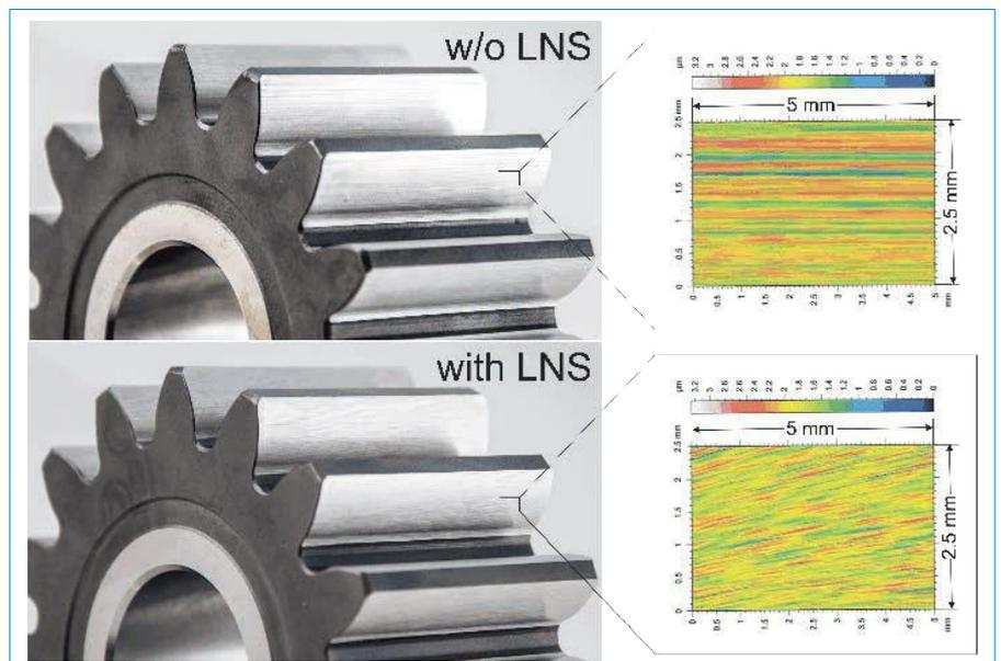
Figure 3 Surface structure w/o and with LNS
