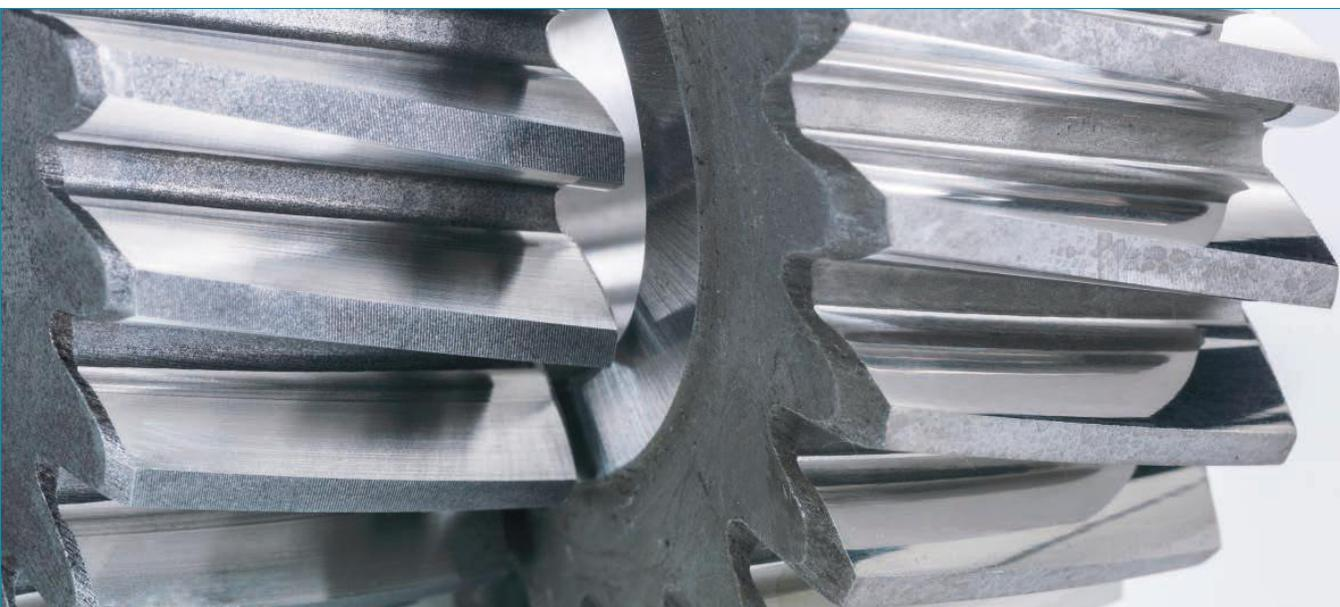
Figure 5 Ground and polished gear flanks
