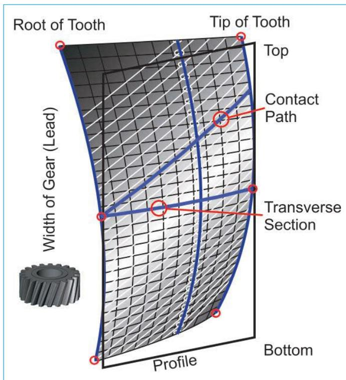
Figure 6 Twist on individual gear flank
