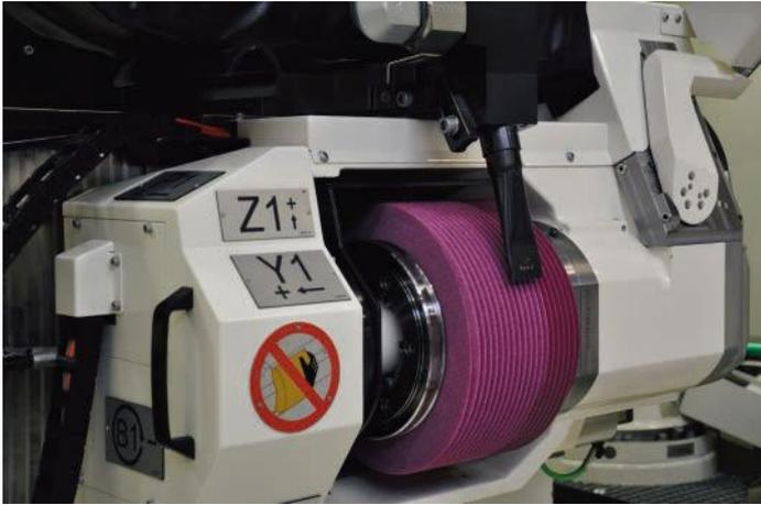
Figure 4 Two-zone grinding worm (Grinding & Polishing)
